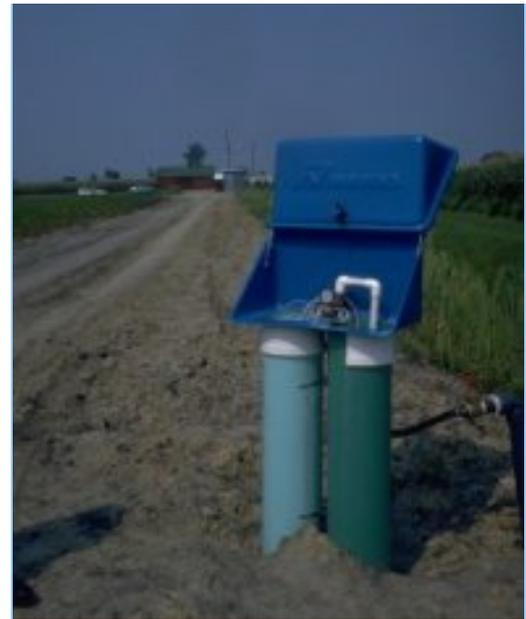
Sub-irrigation and controlled drainage provide water to plants from below the root zone.
