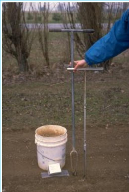
The physical properties of your soils must be known to help make irrigation scheduling work effectively. The technician in this case is taking soil samples to measure water-holding capacity.
