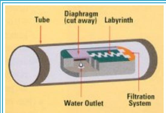
In-line emitters like this can be designed with pressure-compensating features that help maintain the same discharge rates throughout an irrigated field. Pressure-compensating emitters deliver the same flow rate over a wide range of line pressure. This overcomes the problem of slope and distance from the pump.
