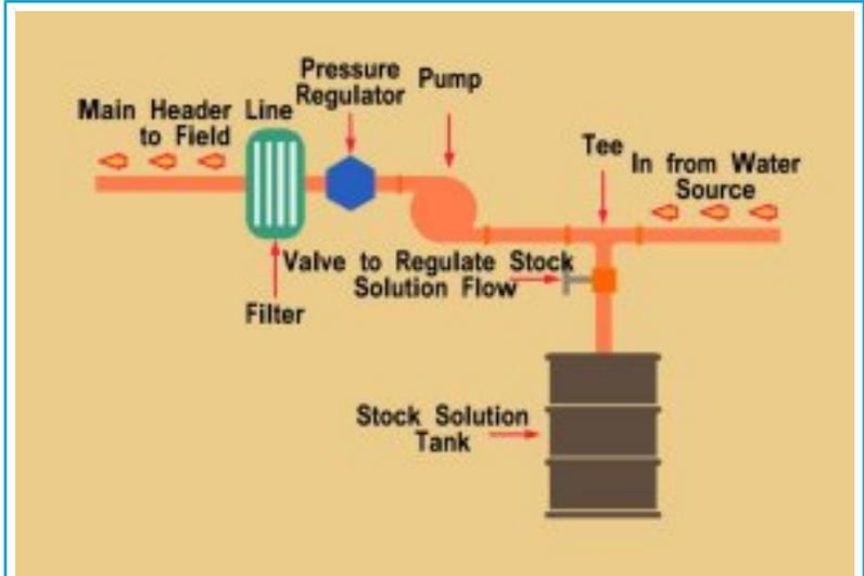
Installing a tee is less expensive, and is usually on the suction side of the irrigation pump. It functions in a fashion similar to a fertilizer injector.
